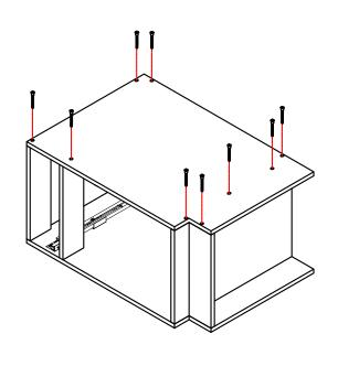
The other side panel is also assembled with the screw
